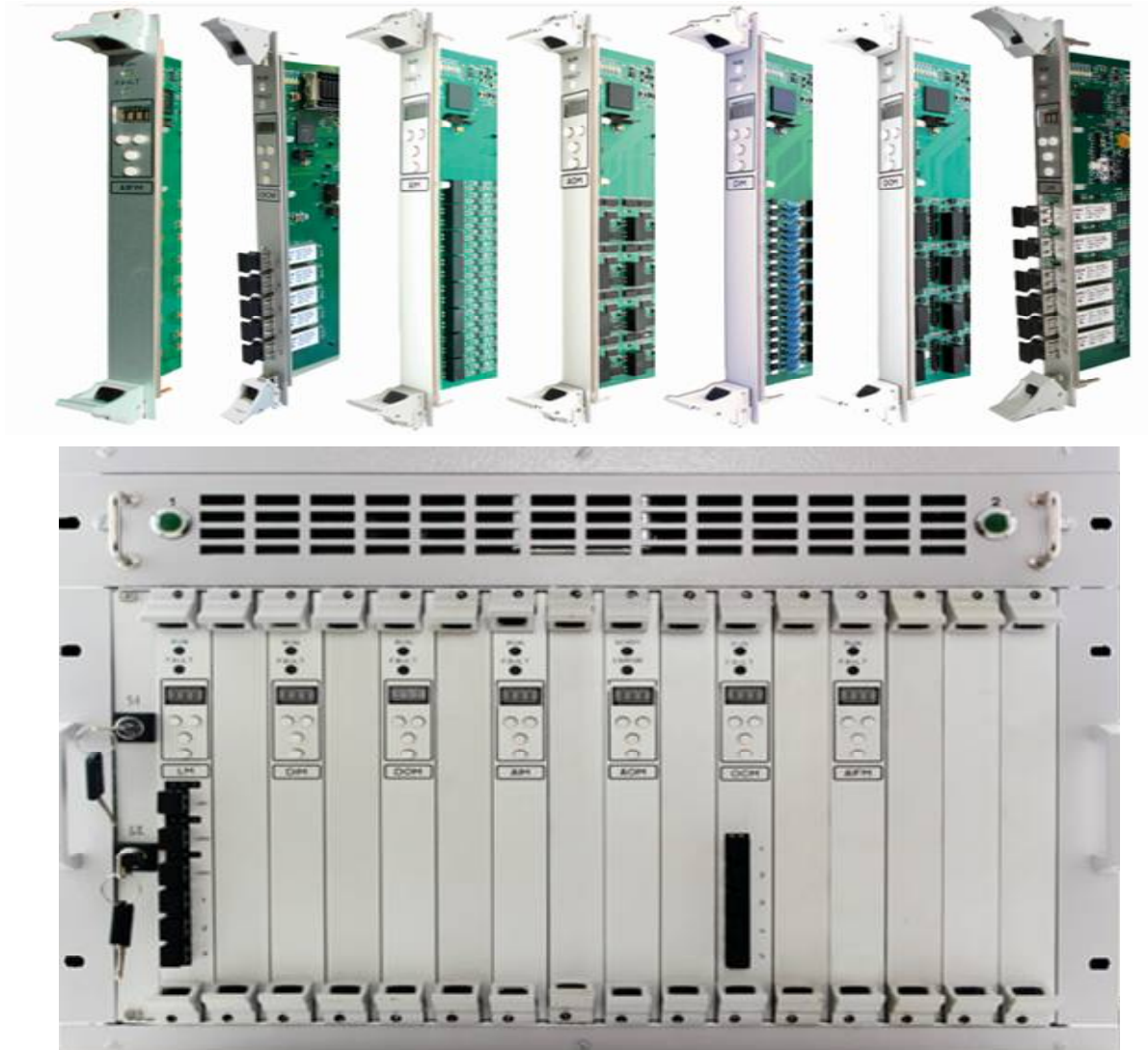
Figure 1. RadICS FPGA-based Platform modules and a chassis with 7 modules inserted.
