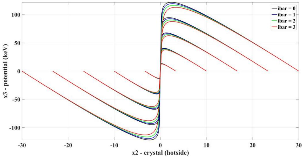
a) Effect of model  $\bar{I}$  operating point variations on crystal temperature-potential trajectories
