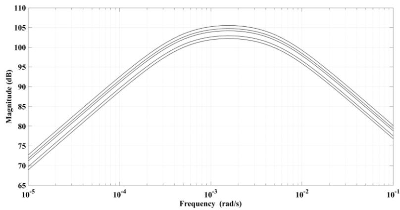
b) Effect of model vacuum chamber temperature  $\overline{T}_c$  operating point variations.
