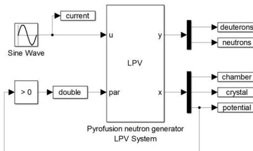
**Figure 5. Example block diagram of a pyrofusion LPV Simulink model.**
