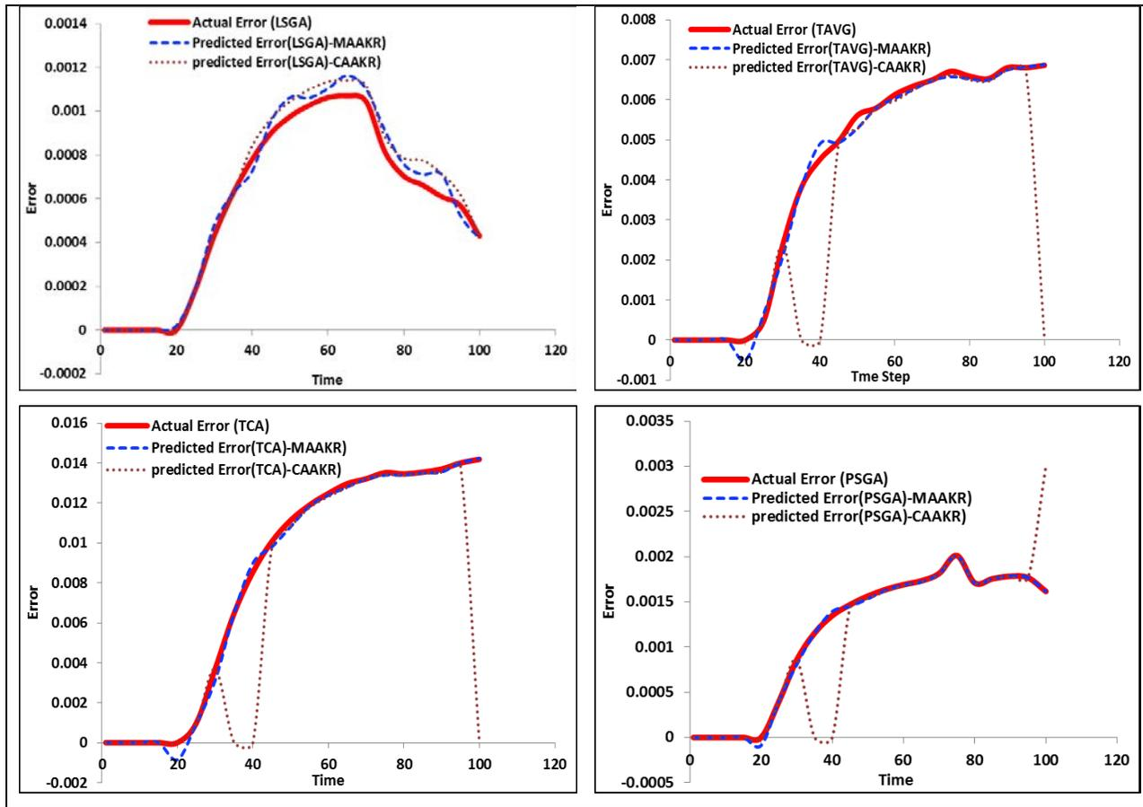
**Figure 5. Residuals plot obtained from the test data that is corrupted as result of LOCA Accident (AAKR)**
