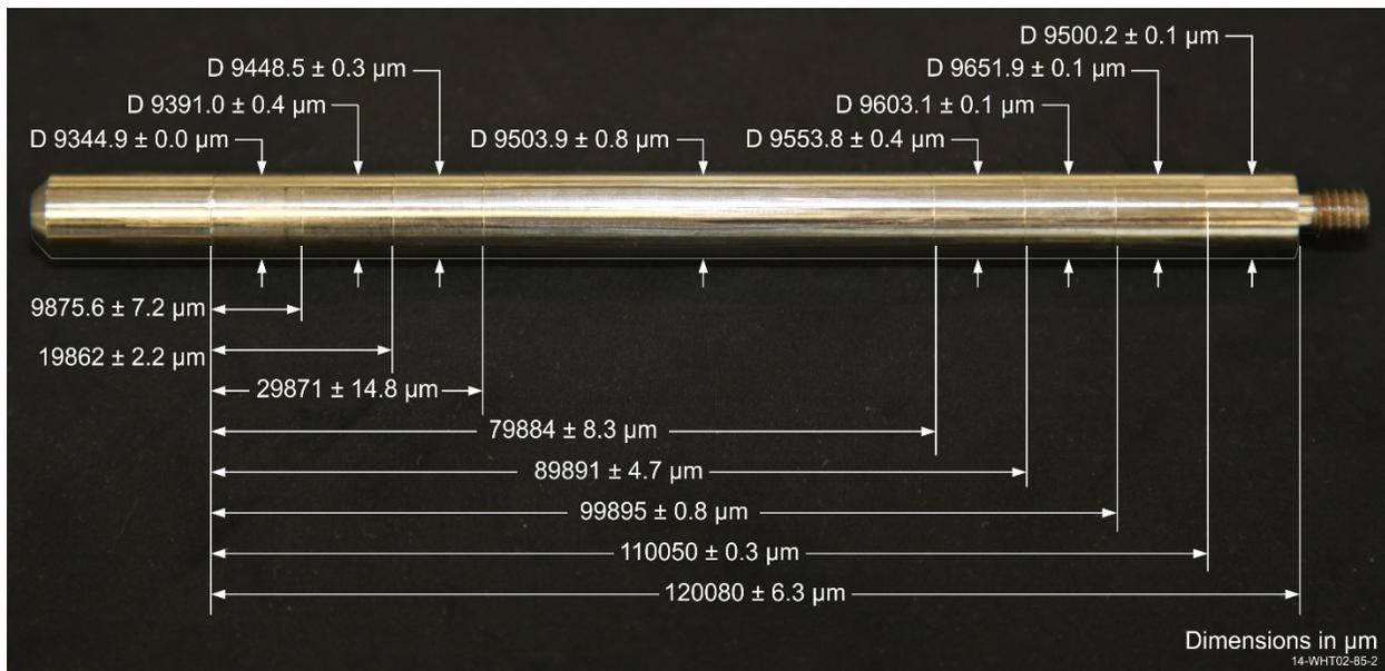
**Figure 4. Test specimen with specific dimensional zones. Metrology information is shown with the measured variances.**
