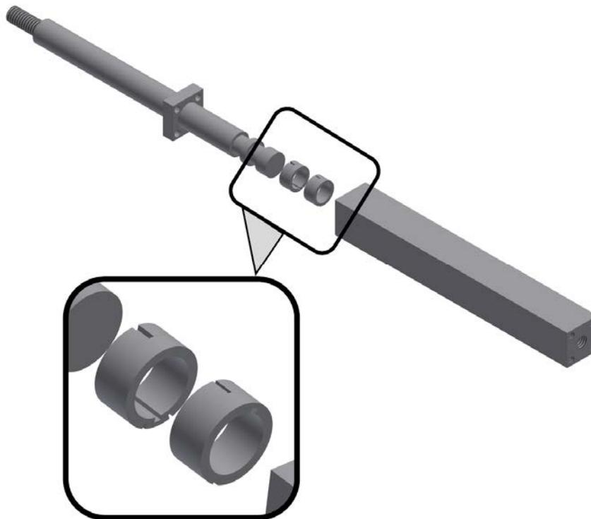
Figure 3. Piston cylinder assembly with zoomed view of piston ring interaction.
