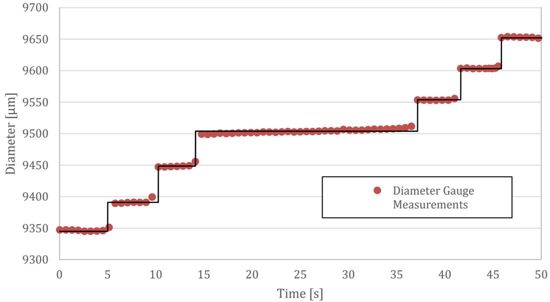
**Figure 5. Results from the Diameter Gauge apparatus on the benchtop scale at a constant rate of 2.2 mm/sec.**
