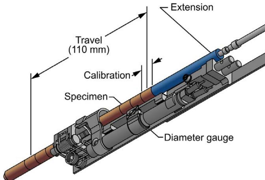
Figure 2. Conceptual design of INL-designed diameter gauge test rig proposed for ATR.
