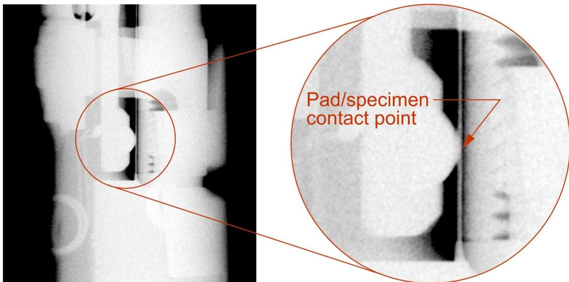
**Figure 6. Radiograph of specimen inserted into diameter gauge.**
