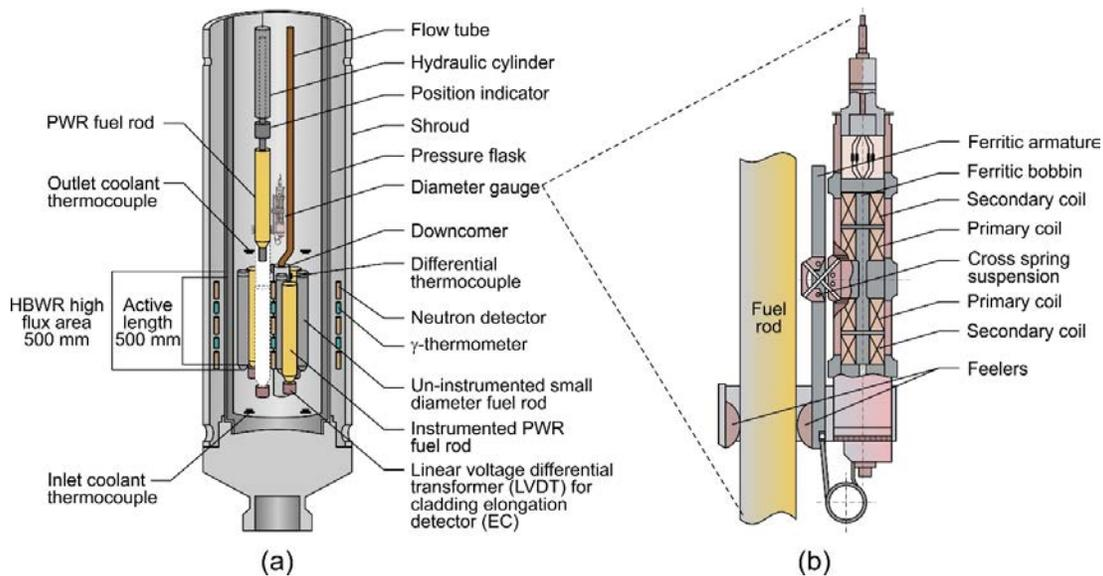
**Figure 1. IFE fuel pellet cladding mechanical interaction/crud deposition test rig (a) with diameter gauge (b) [3, 4].**
