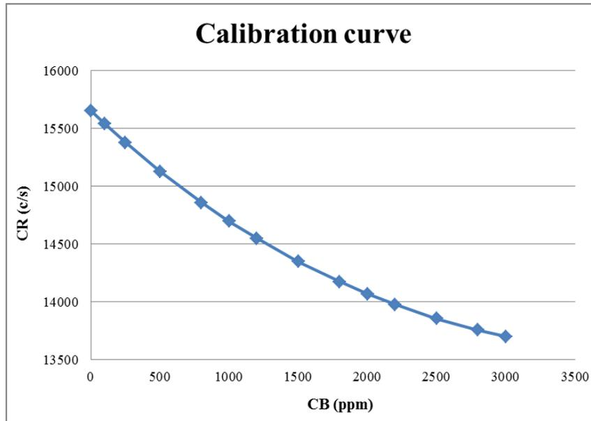
**Figure 2: Calibration curve, or the negative correlation between counting rate and Boron concentration**
