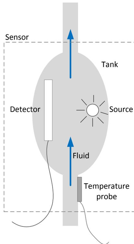
**Figure 1: Measuring principle of a boron meter**
