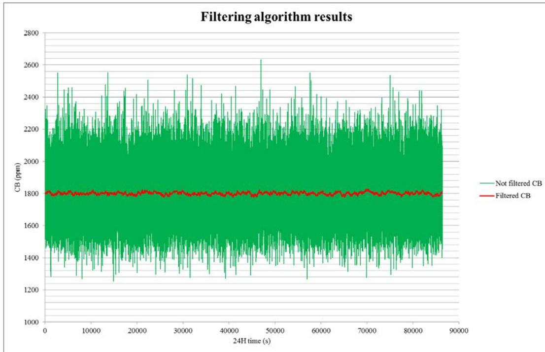
Figure 5: Boron concentration output before and after filtering (24H data recording)
