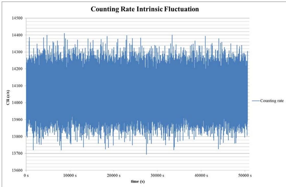
**Figure 3: Counting rate intrinsic fluctuation (24H data recording)**
