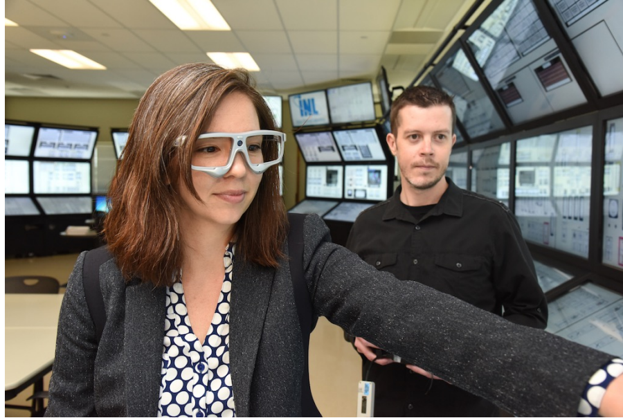
Figure 1. Illustration of a wearable eye tracking system used during a full-scale simulator study.
