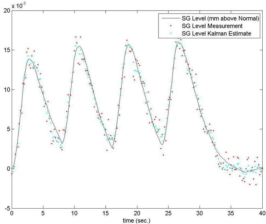
**Figure 5. SG Level with Kalman Estimate**
