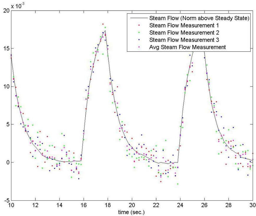
**Figure 3. Steam Flow with Noisy Measurements**
