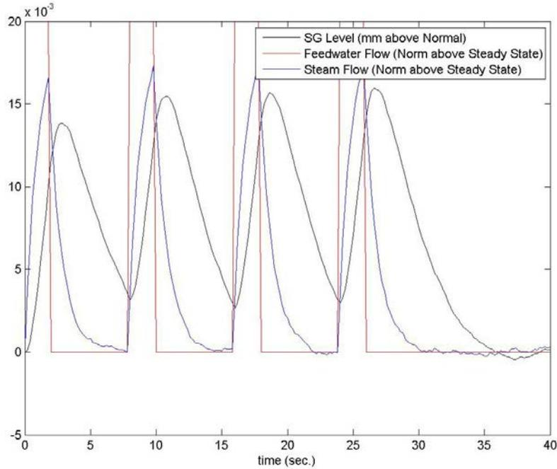
**Figure 1. FW Flow, Steam Flow, and SG Level**
