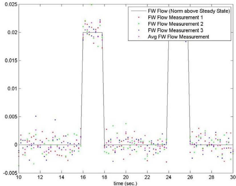
**Figure 2. FW Flow with Noisy Measurements**
