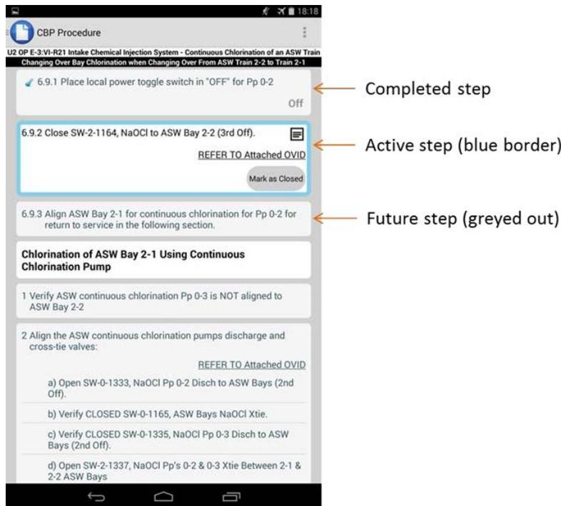
Figure 2. Example of completed step, active step, and future steps.
