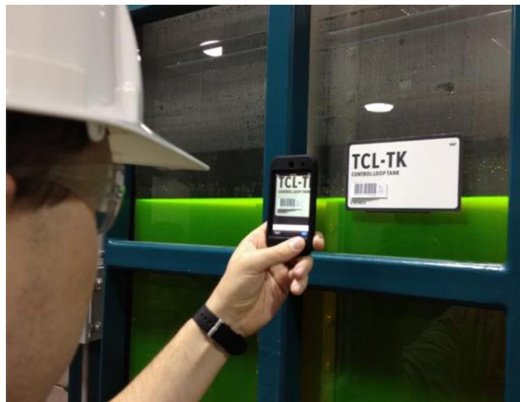
**Figure 5. A field worker conducts a CCV using a barcode scanner.**
