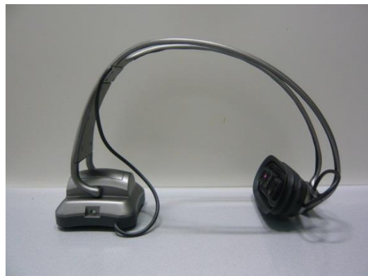
Figure 1 Ultra-small single channel wireless NIRS device (HOT05)
