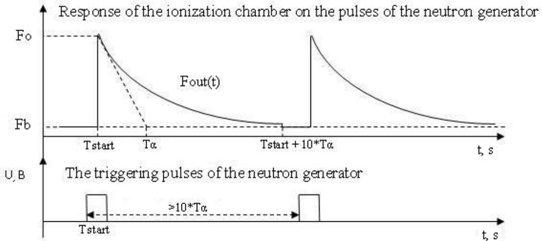
**Figure 3. Timing diagram of the signals, simulating the fission chamber response**
