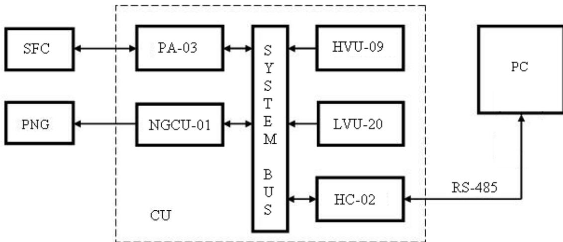
**Figure 1. Measuring system block diagram**
