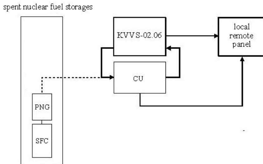
**Figure 4. Block diagram for calibration and verification**
