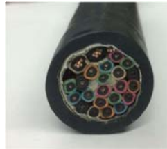
Figure 1. Cross section of BIW control rod cable.
