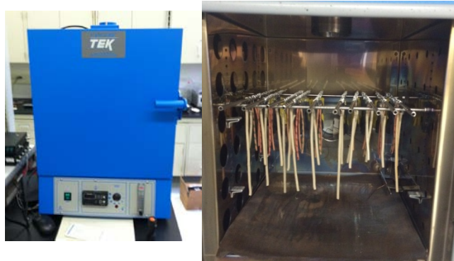
Figure 4. Example of furnace (left) and sample arrangement (right) utilized in accelerated thermal aging of BIW cable and jacket samples.
