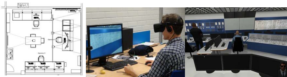
Figure 2. Layout of the physical room space in which the validation test was organized, VR workstation setup and first person view of shift supervisor in the VR CR
