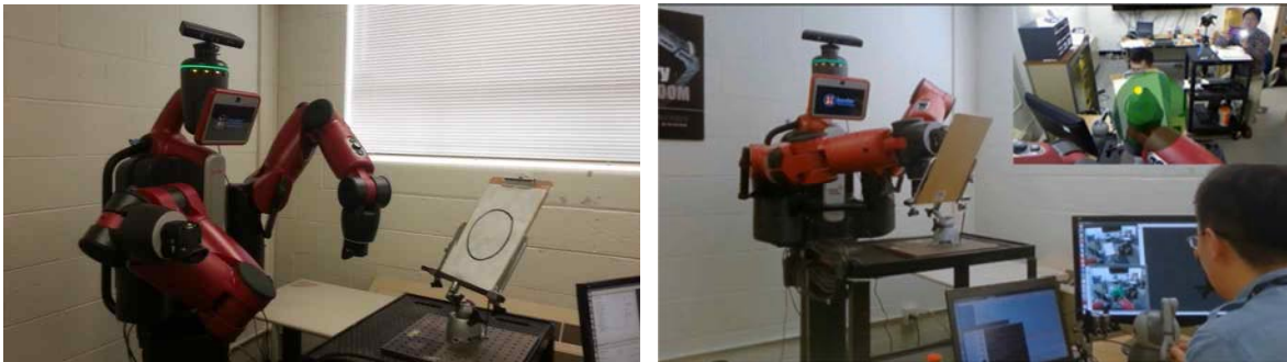
Figure 13. Teleoperation Test Setup with a Circular Pattern
