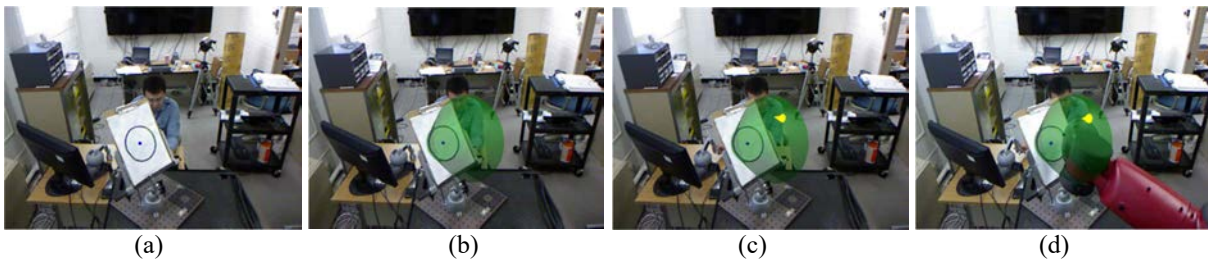
Figure 8. Implementation of virtual fixture for guiding in telerobotic operation. (a) Live image captured by Kinect camera, (b) Virtual fixture placed, (c) Haptic stylus interacting with virtual fixture, (d) Robot arm guided by virtual fixture
