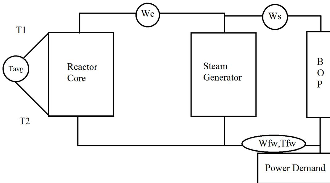
**Figure 4.** Diagram of reactor systems and PID controls.
