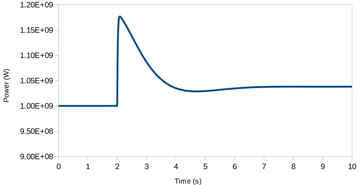
**Figure 5.** Step reactivity insertion of  $+0.001 = 15.4\text{¢}$  yields 4% power increase, in agreement with the NERI-C report from the University of Tennessee [5]. Cold leg temperature is fixed at  $292\text{ °C}$ .
