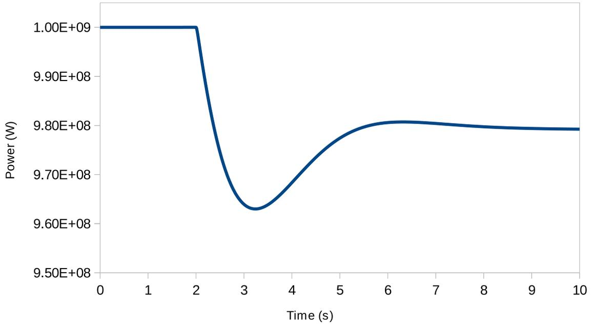
**Figure 6. Step cold leg perturbation of +0.75°C.**
