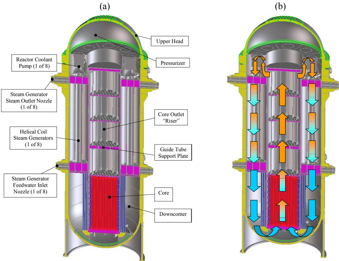
**Figure 1. IRIS integral layout: (a) main components; (b) main flow path [1]**
