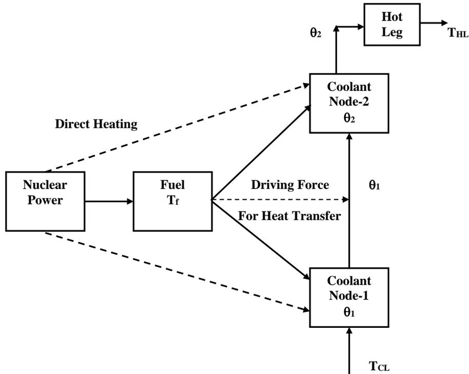
Figure 2. Mann's model of heat transfer between fuel node and coolant nodes [5]
