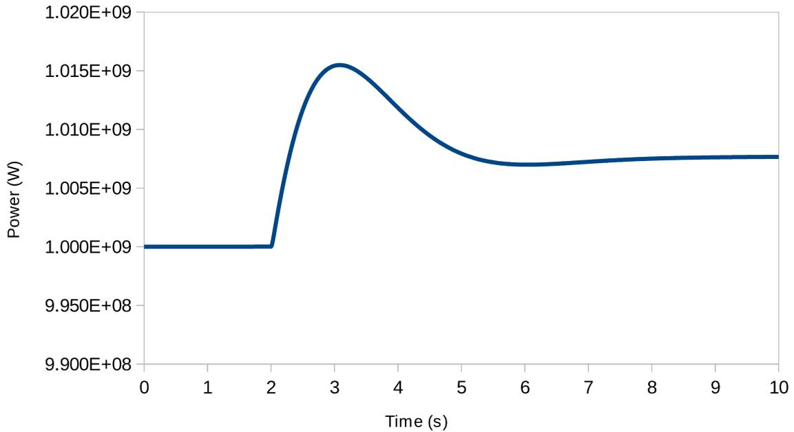
**Figure 7. Step coolant mass flow rate perturbation of +1%.**
