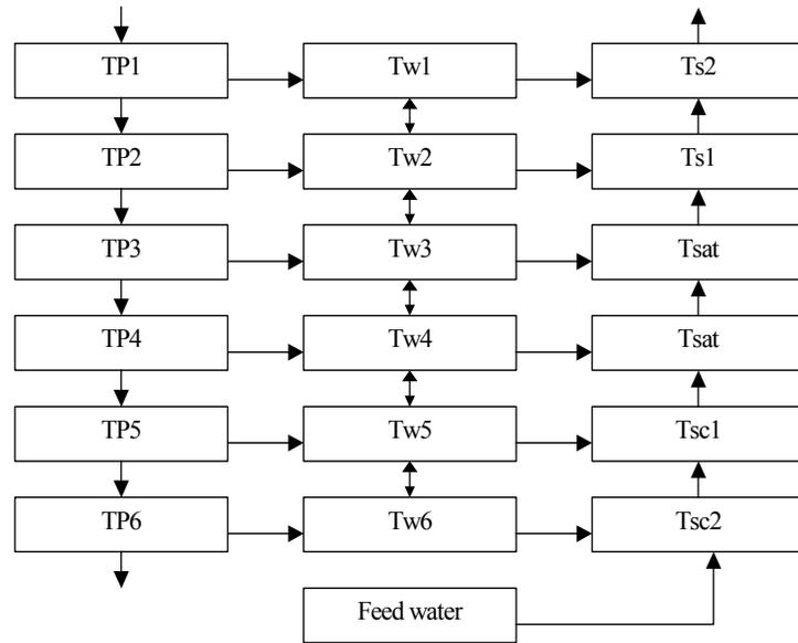
**Figure 3.** Nodalization of steam generator into primary loop, tube wall, and secondary loop [8]. The inlet temperature TP1 is the hot leg temperature of the reactor core, and the outlet temperature TP6 is the cold leg temperature of the core.
