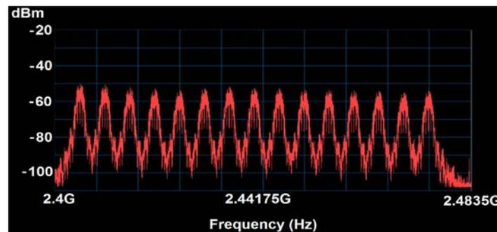
**Figure 2. WirelessHART Channels on 2.4 GHz ISM Band**
