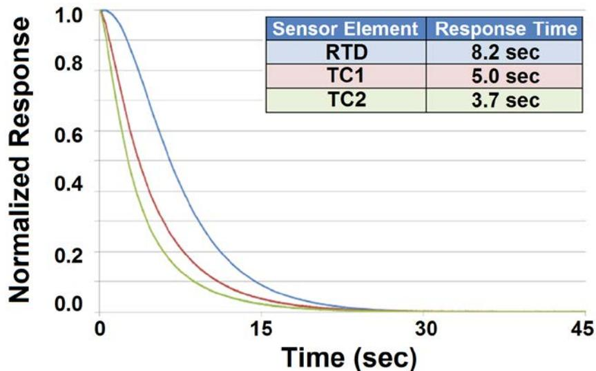
**Figure 4. Plunge Test Data and Response Time Results for TTS Probe**
