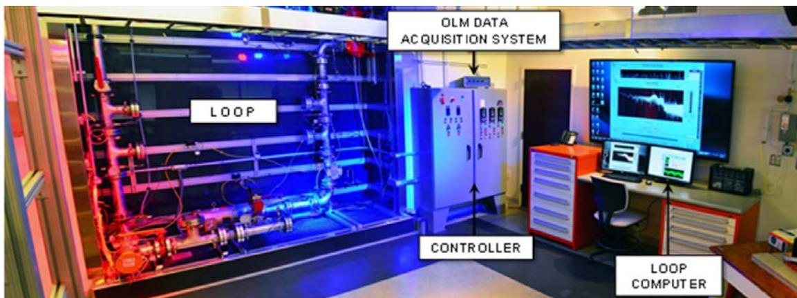
Figure 1. AMS Flow Loop Test Facility
