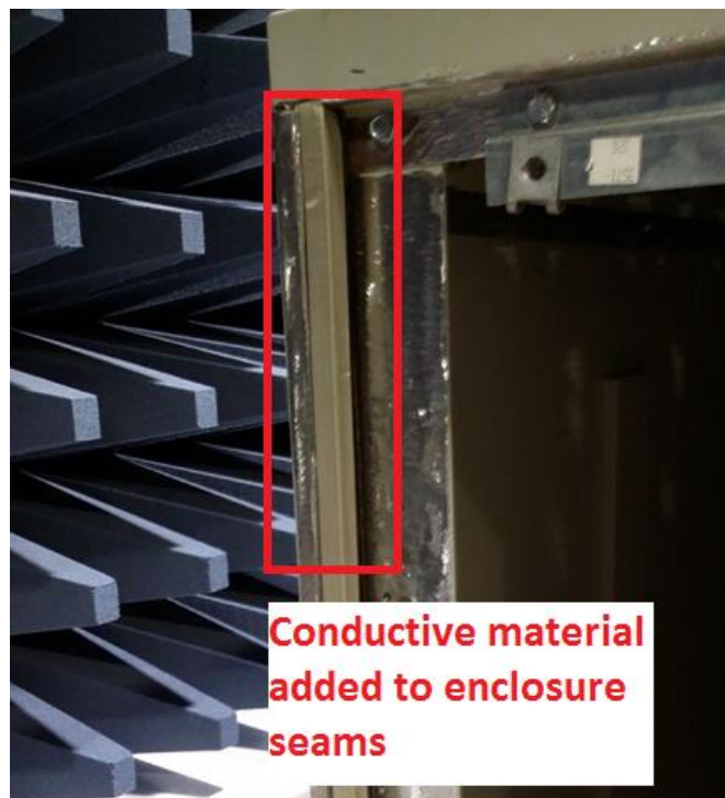
Figure 6. Application of EMI gasket to a 7.5 kVA inverter enclosure
