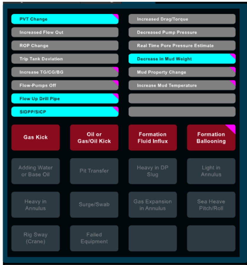
Figure 1. Prototype Delphi design for evaluating alternative explanations in deepwater drilling loss of well control events.
